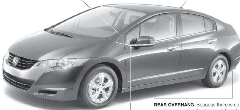
**REAR OVERHANG** Because there is no gasoline engine under the hood, Honda designers were able to give the FCX a short nose. But a large hydrogen tank behind the seats dictated a relatively long area behind the rear wheels.
