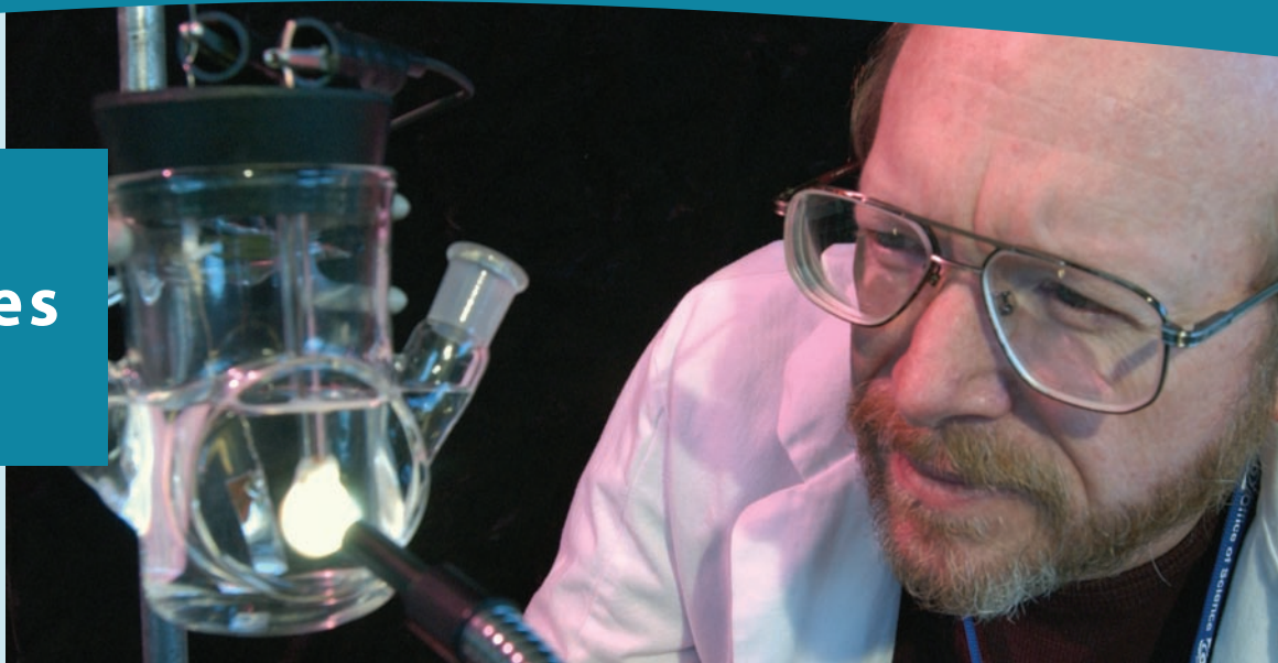
Photoelectrochemical water splitting: Using a photovoltaic cell/electrolyzer submerged in an alkaline aqueous solution to produce hydrogen. Richard Peterson/PIX12958
